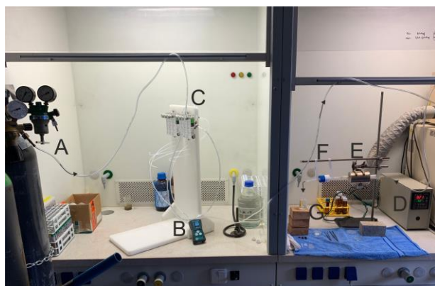
Fig. 2 Experimental combustion set-up. A) synthetic air flow, B) flow meter no.1, C) flow meter with precise regulation, D) temperature regulation, E) horizontal resistance oven, F) PTFE filtering unit, G) capturing acid at the output.
